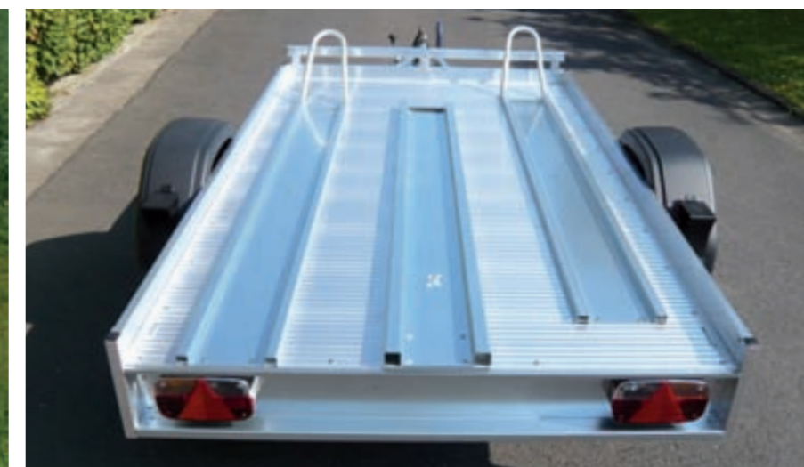
Mot 1025/151 2 galvanised-steel motorcycle stands, 1 loading ramp
